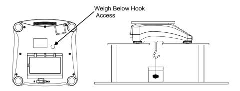
Figure 3-5. Setup for the Weigh Below Hook
