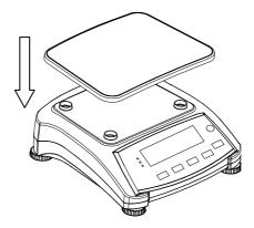
Figure 2-1. Installing the pan
