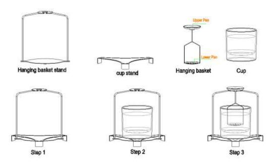
When weighing in air, place the sample on the upper pan of the hanging basket.
